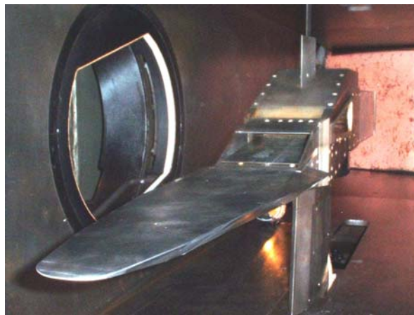
Fig.5 – Mach 2/Mach 8 variable geometry air inlet tested in ITAM wind tunnel
